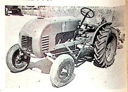
Capacity: Two 14" plows. Performance: Not yet tested at Nebraska Engine: Jeep Model 1949, L-head, 4 cyliders vertical, 31/8x13/"—2000 rated rp
